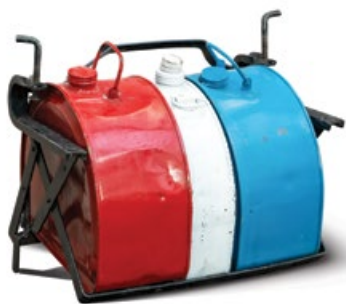
FORD MODEL T ACCESSORY GAS, OIL, AND WATER CANS WITH MOUNTING RACK
